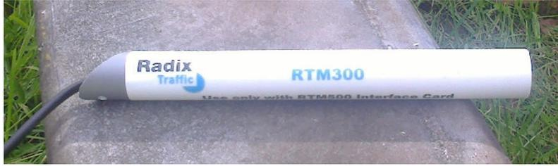
Figure 8 Radix Magnetometer Detector
